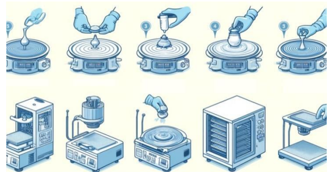
Figure 1 Schematic diagram of Liquid Silicone Spin Coating and Heating Curing preparation process
