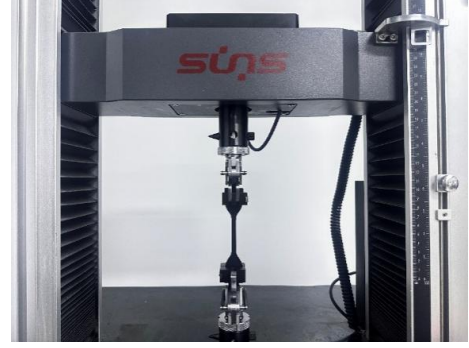
Figure 8 Uniaxial Tensile Test
